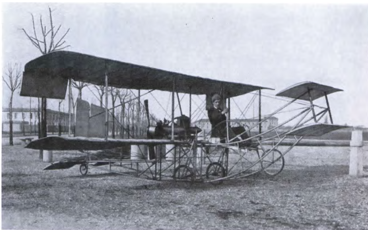
The Faccioli N.4 aircraft was originally powered by the SPA-Faccioli N.2 engine. In 1911, the eight-cylinder SPA-Faccioli N.3 engine was installed. This image was taken in June 1911, with the N.3 engine installed and Mario in the aircraft.
